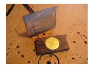
Cover with a laminate. I used a larger piece so that I could sand down.
