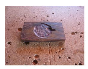
I used a dremel tool here, but use whatever you have that will do the job. You don't need to worry about exact depth as we will "float" the piezo on a bed of hot glue. The dips you see are the solder points on the piezo. The outside dip is for the wires.
