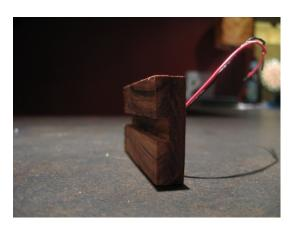
Create the bridge channel. You can either route a channel, or glue on two side pieces as I've done here.
